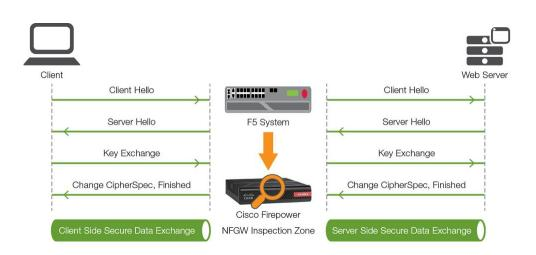
Figure 1: The F5 full proxy architecture.
