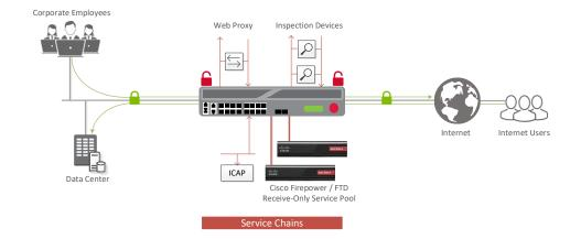
Figure 12: A TAP service deployment architecture.
