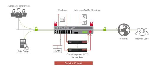
Figure 5: A sample L2 service deployment architecture.
