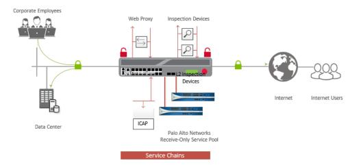
Figure 11: A TAP service deployment architecture.
