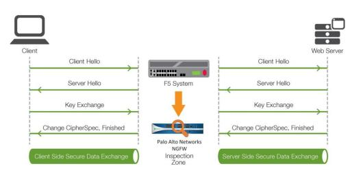
Figure 1: The F5 full proxy architecture.
